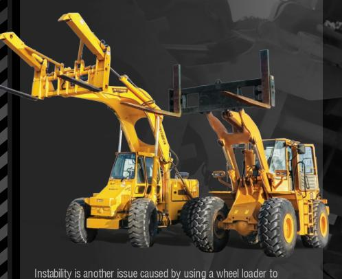
A wheel loader can lose up to half of its rated load capacity when going into a turn. At best, a driver will have to resort to inefficient multiple-point turns. At worst, the machine will tip over. Unfortunately, a wheel loader lying on its side with pipe scattered
